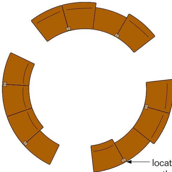
location of undermounted power outlet, typical for 2 at each piece
